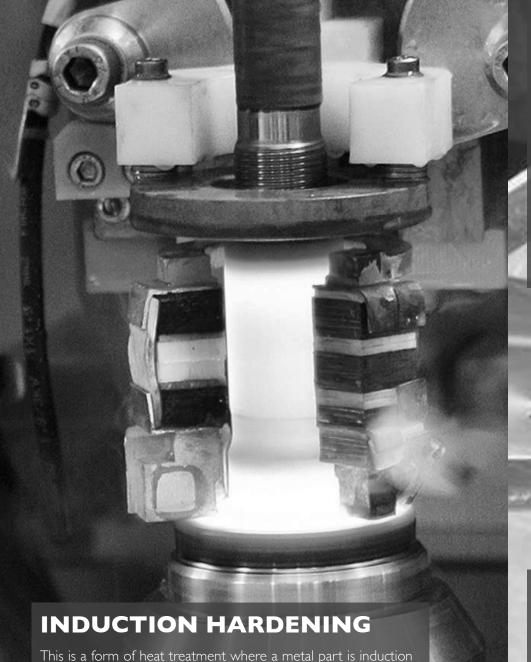
heated and then hardened. The tempered metal then undergoes martensitic transformation for the part to become harder and
